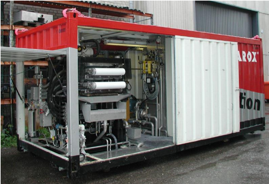
Figure 14. Larox PF 1.6 container unit.
